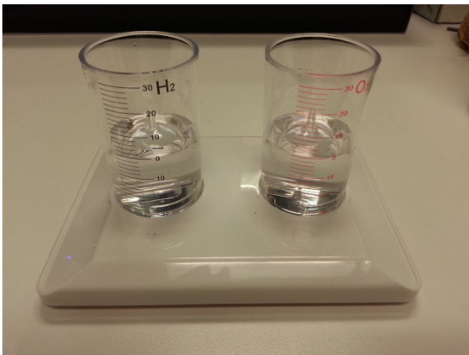
Figure 4: Gas collection cylinders with distilled water levels equal to 0.
