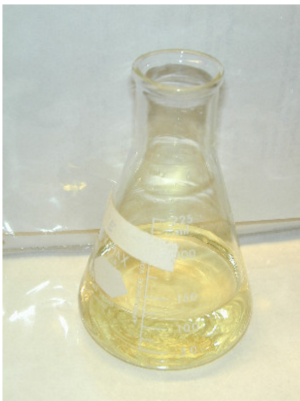
Figure 3. A sample after addition of sodium thiosulfate displaying a pale straw color.
