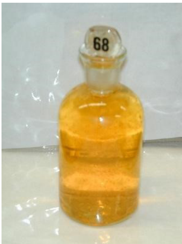
Figure 2. A sample with dissolved floc after addition of sulfuric acid.
