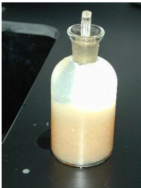
Figure 1. A sample after the alkaline iodide-azide reagent has been added and mixed, showing floc formation at the top of the sample before settling.
