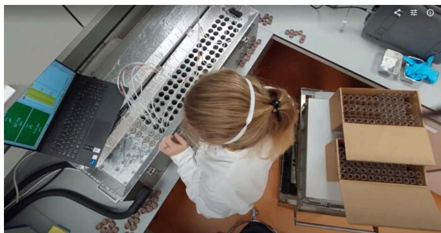
Figure 11: Loading temperature gradient block setup. Please click here to view a larger version of this figure.
