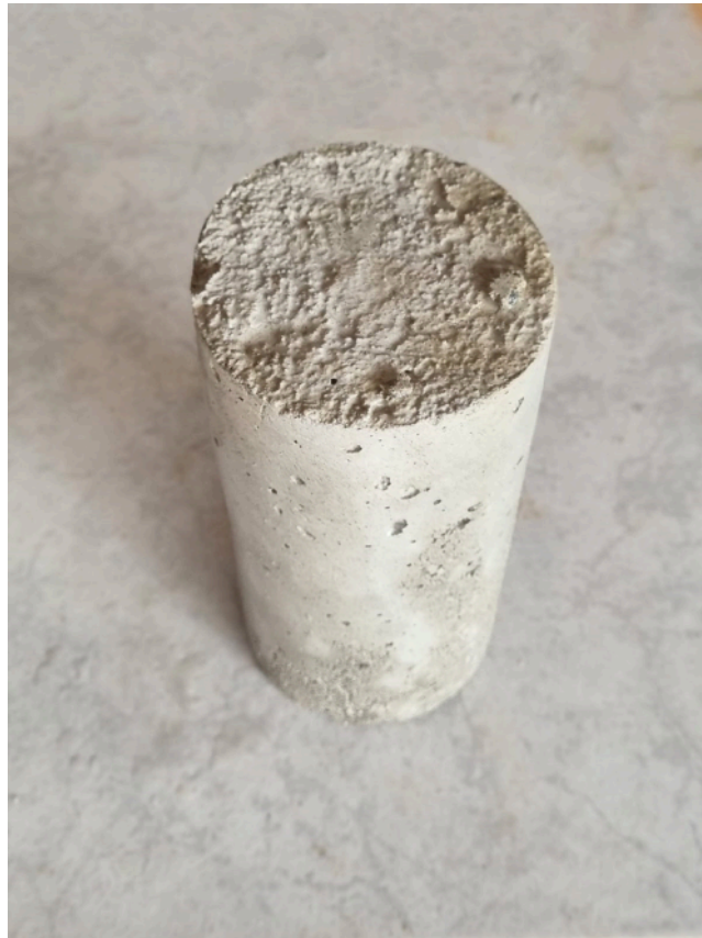
Figure 1: Cylindrical concrete test specimen molded according to ABNT NBR 5739. Please click here to view a larger version of this figure.
