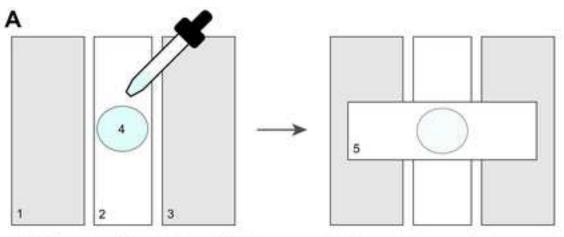
1 & 3: Glass plate of 2 mm thickness; 2 & 5: Microscope slide of 1 mm thickness; 4: 2% Agarose pad
