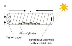
"(A) Illustration of artificial feeding chamber. The cylinder is 15.0 cm long and 2.5 cm in diameter. At one end of chamber is the Parafilm membrane sandwich, the other end, as well as the cylinder wall is covered with tin foil paper (slanted lines) represent the device is covered with tin foil paper. Set the light source to attract SBPH to feeding the artificial diet."
