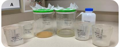
3.6 Heavy liquid isolation of quartz grains, using non-toxic heavy liquid Sodium Polytungstate (SPT-Na<sub>6</sub> ( $H_2W_{12}O_{40}$ )\_ $H_2O$ ).
