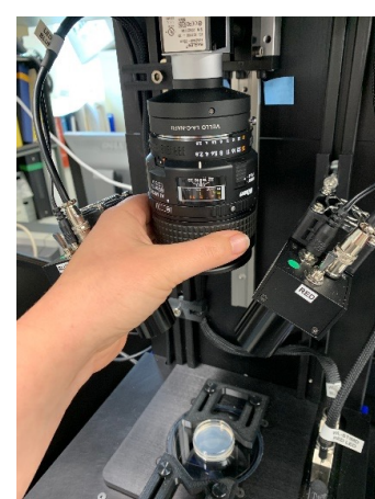
Adjust Focus Ring on Camera Lens as Needed
