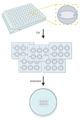
Final PDMS positive plate generated from negative PU mold
