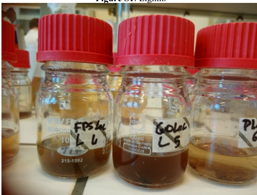
Figure S2: Samples after being autoclaved (30 mg of lignin + 1 mL of 72% sulfuric acid + 28 mL of distilled water).
