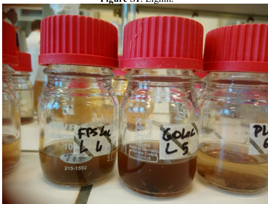
Figure S2: Samples after being autoclaved (30 mg of lignin + 1 mL of 72% sulfuric acid + 28 mL of distilled water).
