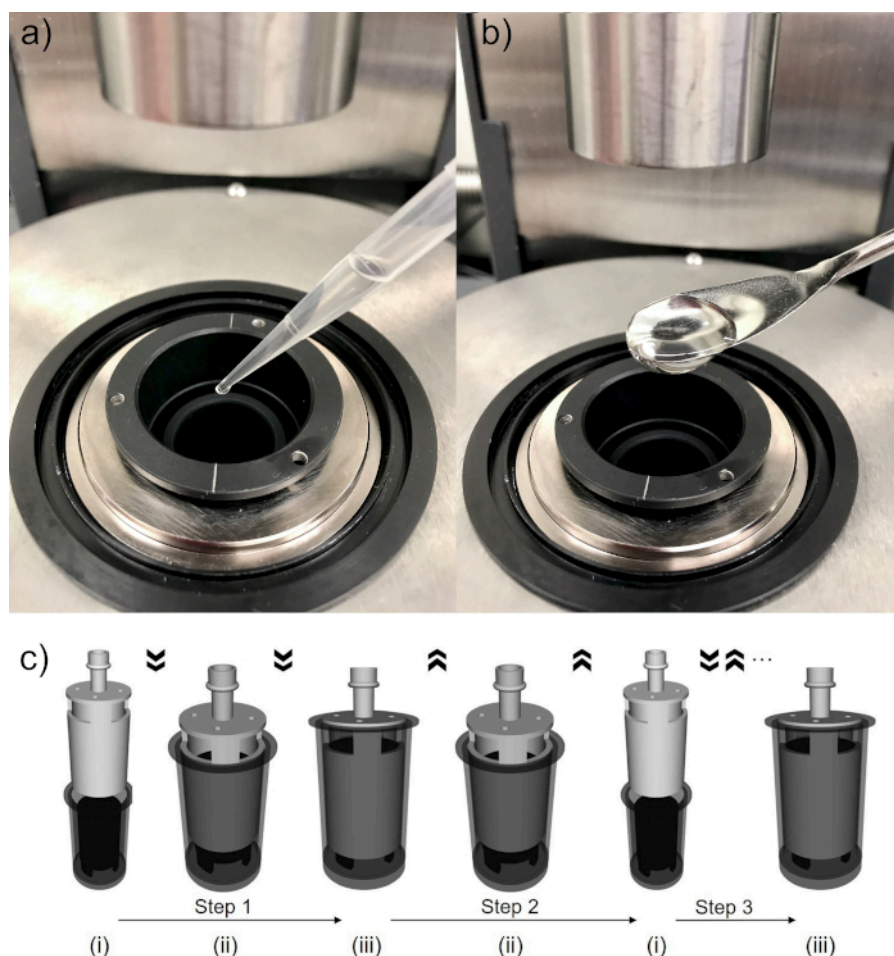
Figure 2: Detailed procedure of loading test materials. (a) Loading a less viscous test material using a pipette. (b) Loading a higher viscosity test material using a spatula. (c) After loading the desired amount of test materials into the cup, slowly insert the bob and decrease the gap to the geometry gap (Step 1); Lift the bob to check the fluid level by examining the wetted contact line (Step 2); Repeat this procedure while adjusting the volume of the test material until the bob is properly wetted (Step 3). See text for details. Please click here to view a larger version of this figure. Please click here to view a larger version of this figure.
