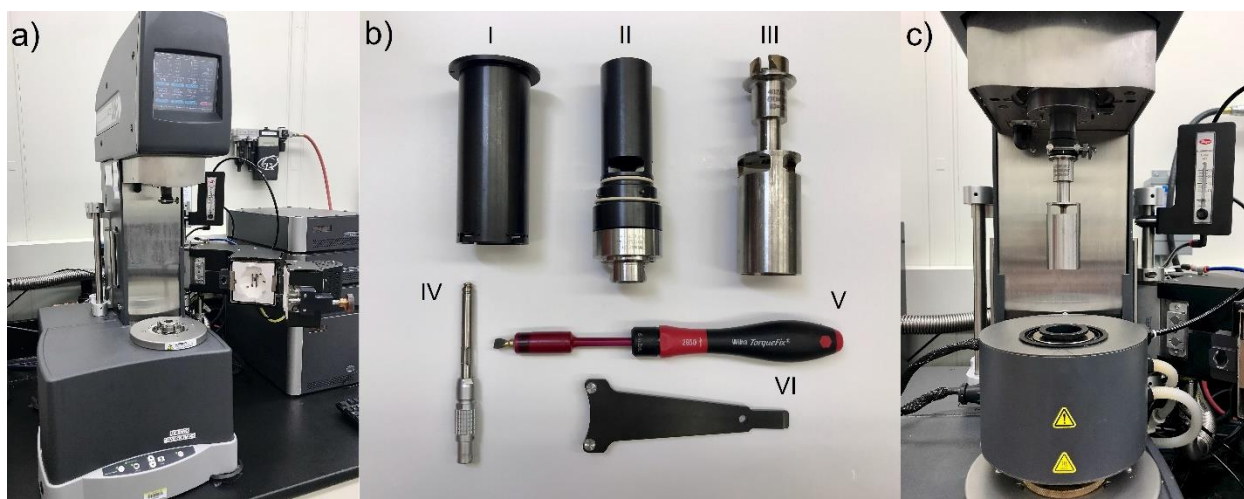
Figure 1: Pictures of the rheometer, the OSP geometry, and the Advanced Peltier System (APS). (a) ARES-G2 test station. (b) Components of the orthogonal double wall concentric cylinder geometry: the outer cylinder (I), inner cylinder (II), and the inner cylinder (III); the PRT (IV), the torque screwdriver (V), and the spanner wrench (VI). See Table of Materials for the part number. The PRT, torque screwdriver, and spanner wrench are included in the APS kit. (c) The rheometer setup after the installation of the environmental control device and the orthogonal double wall concentric cylinder geometry for experiments. Please click here to view a larger version of this figure.
