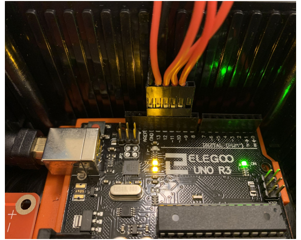
Figure S30: Placement of the crimped wire-to-wire connector. (A) Picture of the crimped wire-to-wire connectors for a four LED-microcontroller system. (B) Placement of the crimped connector into the microcontroller ports.
