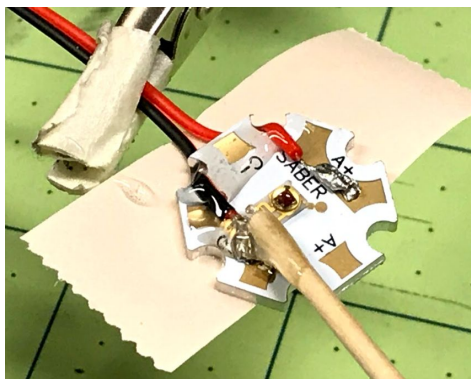
Figure S22: Securing the wires and LEDs to the LED base using epoxy. (A) Using wooden applicator to place epoxy into the LED base. Tape is placed below to catch any dripping epoxy. (B) Epoxy is spread evenly over the entire surface. (C) The LED is left overnight to cure.
