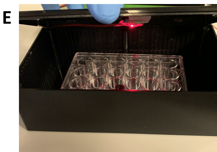
Figure S23: Mounting LEDs inside a box lid. (A) An LED with a command strip piece attached for easy mounting. (B) Different color LEDs mounted on the inside of a black box using a command strip. (C) A notch on the lid of the black box made by a Dremel to make room for the LED wire. (D) A black box for stimulating the cells with touch fasteners for mounting the LED. (E) Placement of a multiwell dish inside of the touch fastener version of the LED box.
