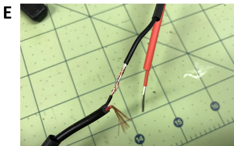
Figure S12: Connecting the power supply to a male wire-to-wire connector. (A) The unmodified power supply. (B) Cutting of the power supply wires. (C) The power supply wires stripped and with excess insulation cut away. (D) Placement of shrink tube around power supply wires. Tubing separating the two connections (red arrows) and tubing to hold the separated wires (yellow arrow). (E) Twisted wires connecting the power supply to the female wire-to-wire connector.
