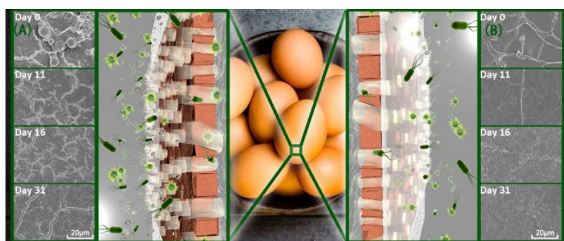
Figure A. SEM images of the raw eggshell surfaces and chitosan treated eggshell surfaces at day 0, 11, 16 and 31 ((a) the raw eggshell surfaces; (b) chitosan treated eggshell surfaces).
