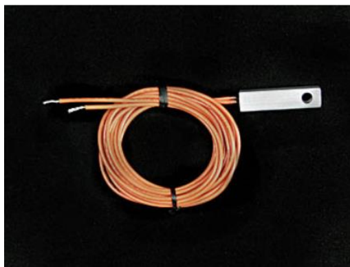
Figure 3: MP-3193 moisture-resistant thermistor. Two leads will be placed in temperature controller ports 1 and 2. The metal thermistor will be placed in ocean simulant. (Image: Courtesy of TE Technologies)
