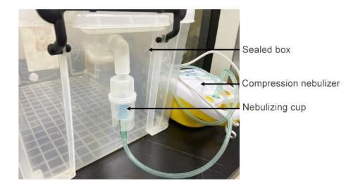
For the detail of the nebulizer can be adapted for small animals: The nebulizing device includes a sealed box, open the lid of the self-made sealed box and place the rat in the sealed box. The corresponding changes have been highlighted in page 6 line 11-15.
