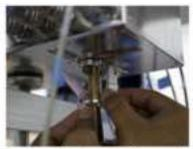
Remove the microcentrifuge tube with the sample catcher as close as possible to the insert/eject line. Insert and tighten the sample catcher.
