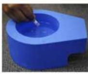
Slide the rotor into the liquid nitrogen bath.
