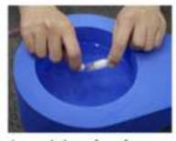
Approach the surface of the liquid nitrogen and unscrew the top of the cryovial.
