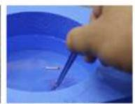
Submerge a microcentrifuge tube using tweezers and hold it in place until it cools down completely.
