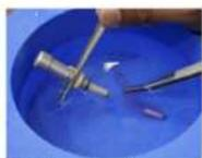
Hold the sample catcher at an angle above the surface and be ready to quickly recover the rotor from the liquid nitrogen.
