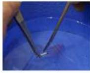
Insert the rotor into the microcentrifuge tube cap forward. Just below the liquid nitrogen We recommend pushing the rotor surface and make sure that the in rather than grabbing it with the tweezers.
