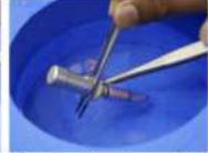
Lift the sample catcher and the tube as soon as the sample catcher is in the microcentrifuge tube.
