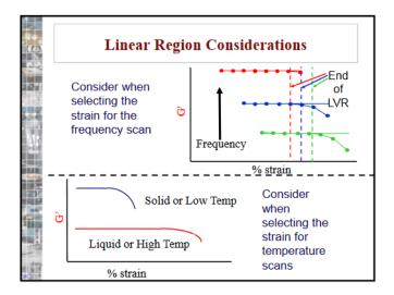
At the minimum temperature the sample is below its glass transition and even taking into account a possible small residual cure, surely the LVR is thinner at the initial temperature.
