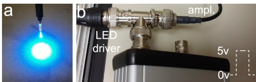
Figure 4: BNC split connection for combined light pulsing and amplifier (trigger) time stamps.
