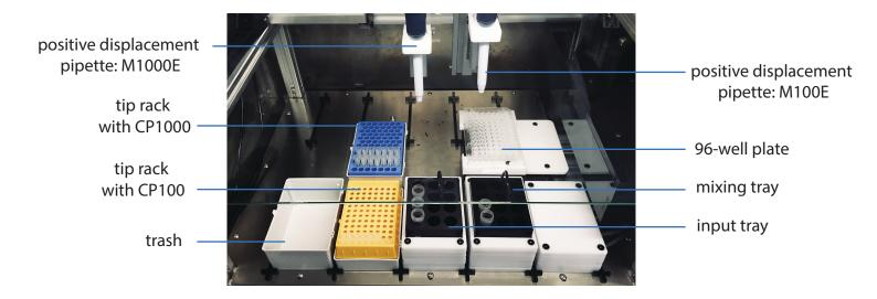
pipetting module: definition of positions
