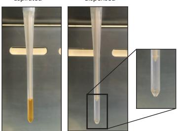
c excess material on tip d tip touch to remove excess material
