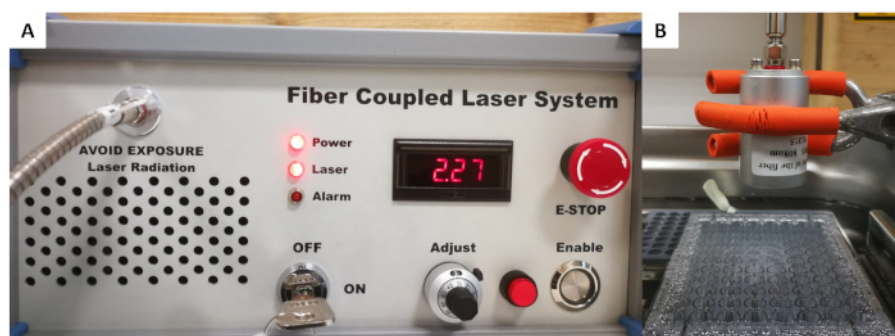
Figure 6: Photograph of the laser setup. (A) Photograph of the fiber coupled laser system during operation. (B) Position of the collimator 5 cm above the 96-well plate. Please click here to view a larger version of this figure.
