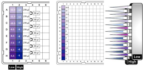
96-well plate for dilution ----- 384-well plate with transfected cells
