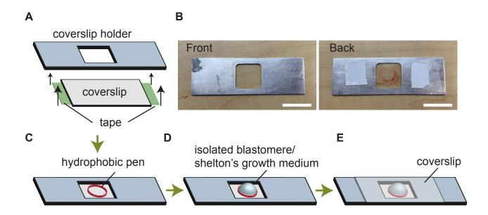
Figure 5. Assembly of imaging chamber
