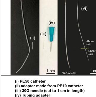
(v) delivery catheter assembly
