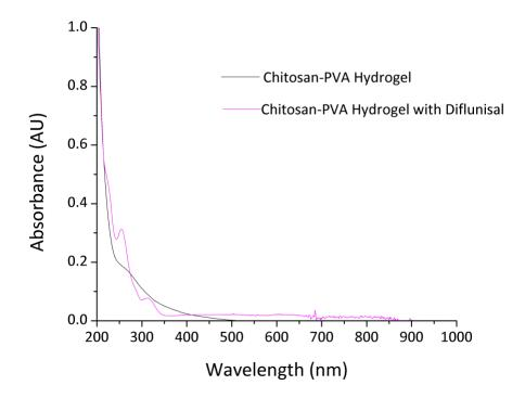
Also, are presented the UV-Vis spectrums obtained during the drug loading studies for one of the sample, were neither interference of hydrogel components was presented.
