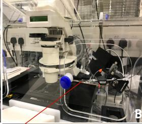
Fluorescence microscope with environmental chamber and microinjection system
