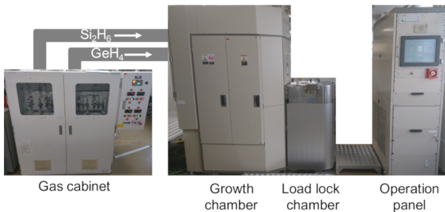
Figure 2: Pictures for parts of an UHV-CVD machine; gas cabinet, process chamber, load lock chamber, and operation computer. Please click here to view a larger version of this figure.
