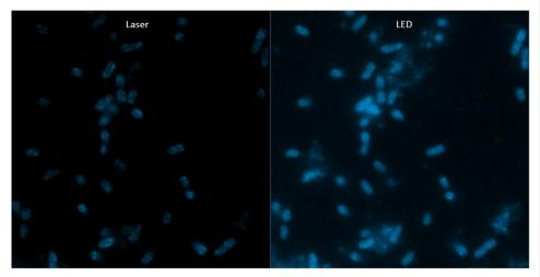
In these two images, the same sample (an inner membrane protein in E.coli cells) area was imaged with exactly same camera condition (100 ms exposure time and maximum gain). The contrast of these images are same so they can be compared side by side. Laser illumination was in Epi mode, with the use of mag lens, to be comparable to LED light.
