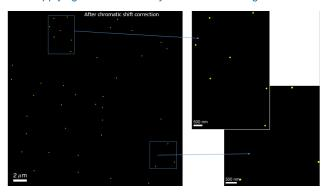
As far as there are these reference samples in the test sample (so immobilize beads to the test sample before imaging), then it is not difficult to align the two channels. Single molecule detection is mostly unaffected, since the beads are not 'too' bright to saturate the pixels, even with high laser powers. Also over time they photobleach too (getting dimmer), making them easier to be picked by the analysis software. We assume they have similar XY resolution since
