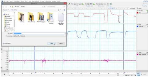
Step 3: Select the flow and  $CO_2$  channels to export, check "current selection" and downsample by a factor of 10
