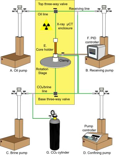
1/8 Stainless steel tubing 1/16 PEEK tubing Thermocouple line Flexible heater line 1/8 to 1/16 converter Two-way valve Three-way valve Three-way connection
