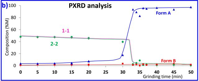
LAG at 30 Hz: Kinetic study equimolar mixture of 1-1 & 2-2 + 2%M dbu +  $50~\mu$ L MeCN
