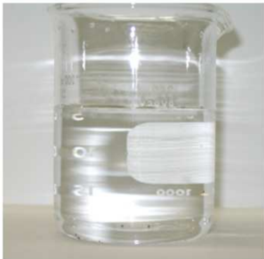
Carbon Nanotubes Before Sonication
