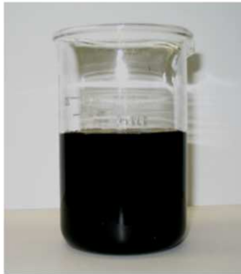
Carbon Nanotubes After Sonication (six months)
