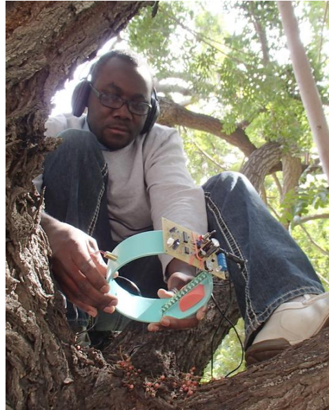
Phytotelmata (small water bodies held by terrestrial plants) are an important breeding ground for many insect vectors. Here a technician is placing one of our sensors over a water-filled tree hollow. The sensor can be left unattended for up to two weeks on battery power.
