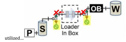
Turning the valves on opens the fluidics pathway extending from the saline
