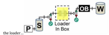
During loading, both valves are set to off, preventing fluid movement as the loader is
