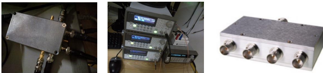
Figure 8 : The generation of radiofrequency signals is performed with a 10 MHz reference clock (a), frequency synthesizers (b) a power splitter/combiner (Minicircuits ZB4PD1-500-75) (d).
