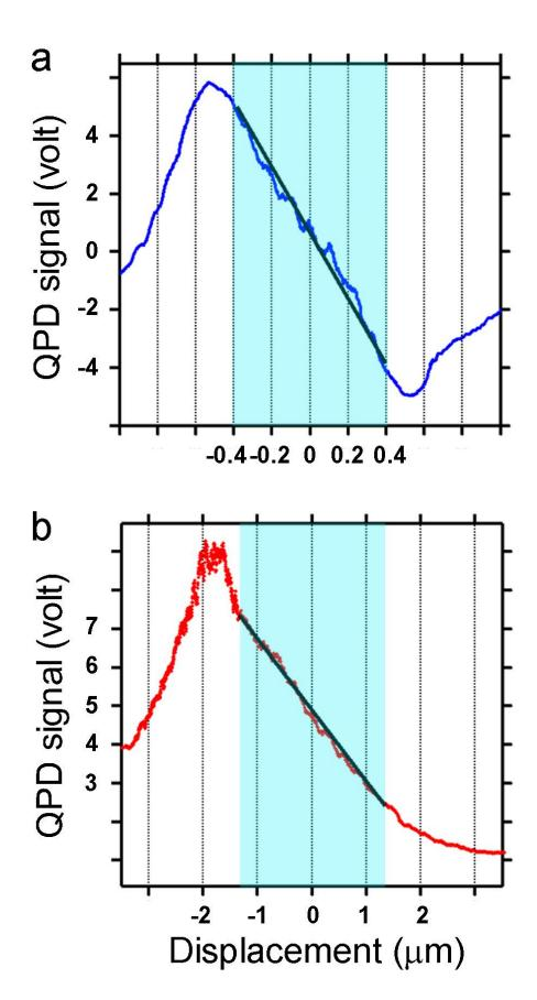
Blue and red traces represent respectively the x and z directions. The bright blue shadow marks the linear range. Standard calibration curves are reported here for reference, but not included in the text.
