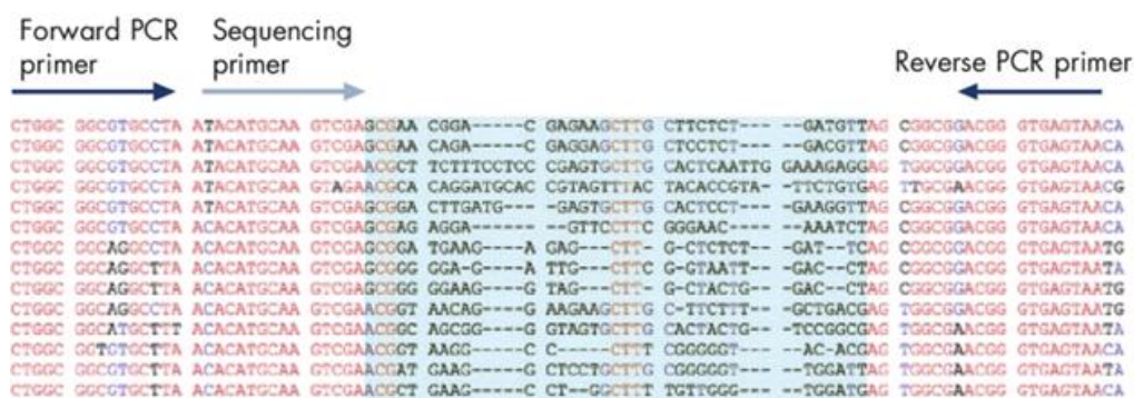
Figure 10: Pyrosequencing based bacterial identification results. PCR primers are designed for conserved regions of the DNA template, and the sequencing primer is positioned immediately upstream of a well-characterized identifying hypervariable DNA sequence within the amplicon (shown in blue).
