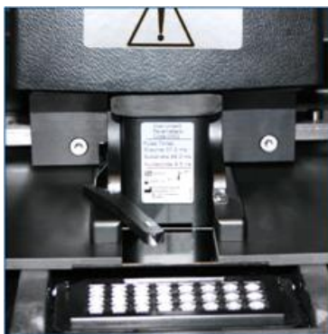
Figure 8. Cartridge gate opened with cartridge in place.
