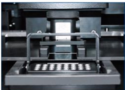
Figure 9. Cartridge properly inserted with gate closed
