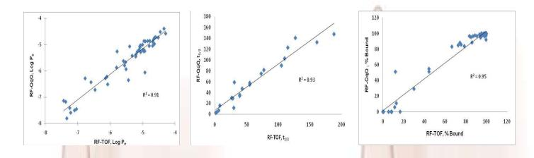
PAMPA, Metabolic Stability and Plasma Protein Binding assays performed with a chemically diverse compound set were analyzed using RapidFire-triple quadrupole(QqQ) MS and RapidFire TOF-MS. The graphs above demonstrate the excellent correlation between data generated using the TOF instrument and that of the QqQ.
