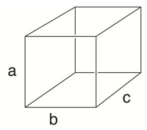
$\alpha$  = angle between b and c  $\beta$  = angle between a and c  $\gamma$  = angle between a and b
