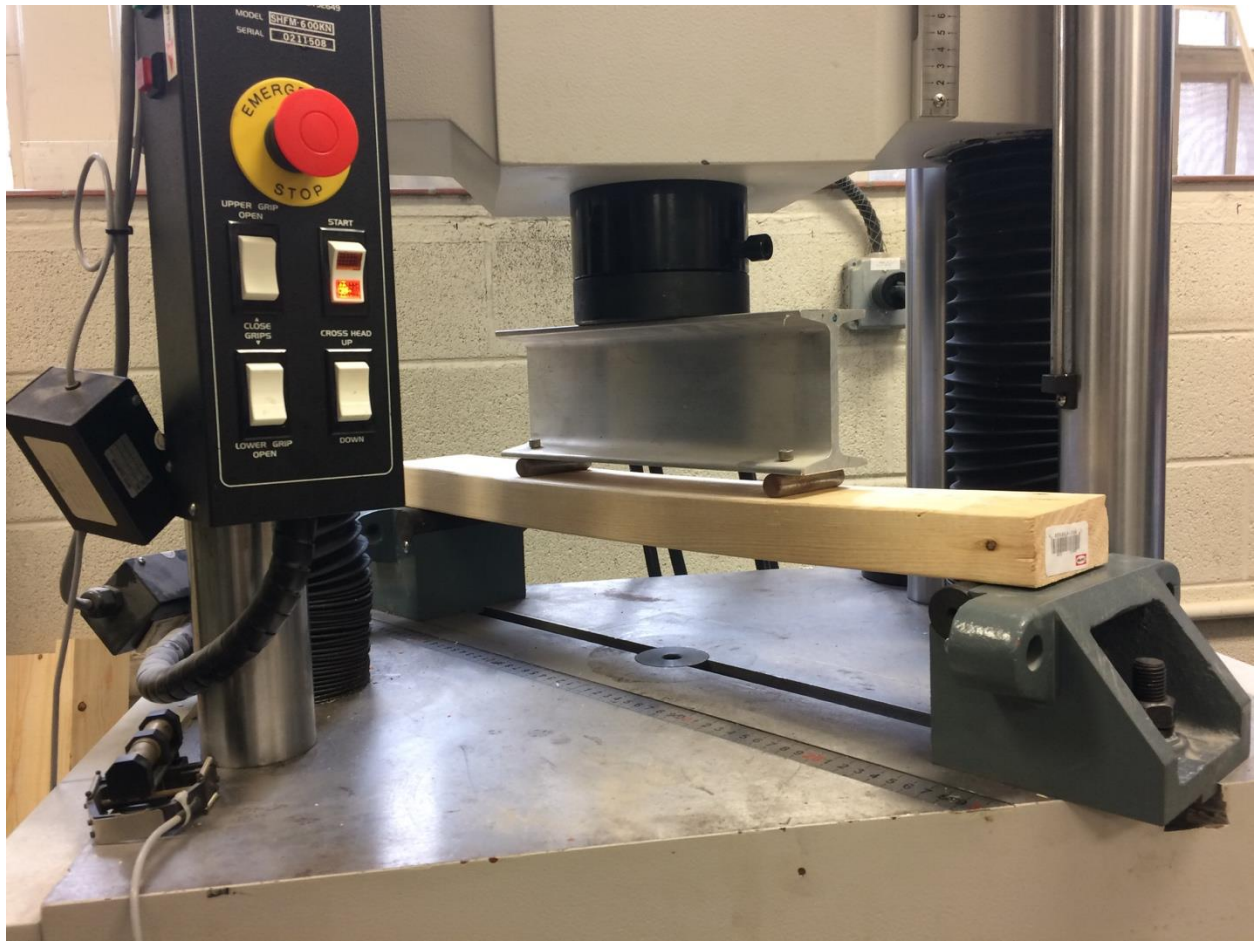
Figure 6 – Four-point bending apparatus
