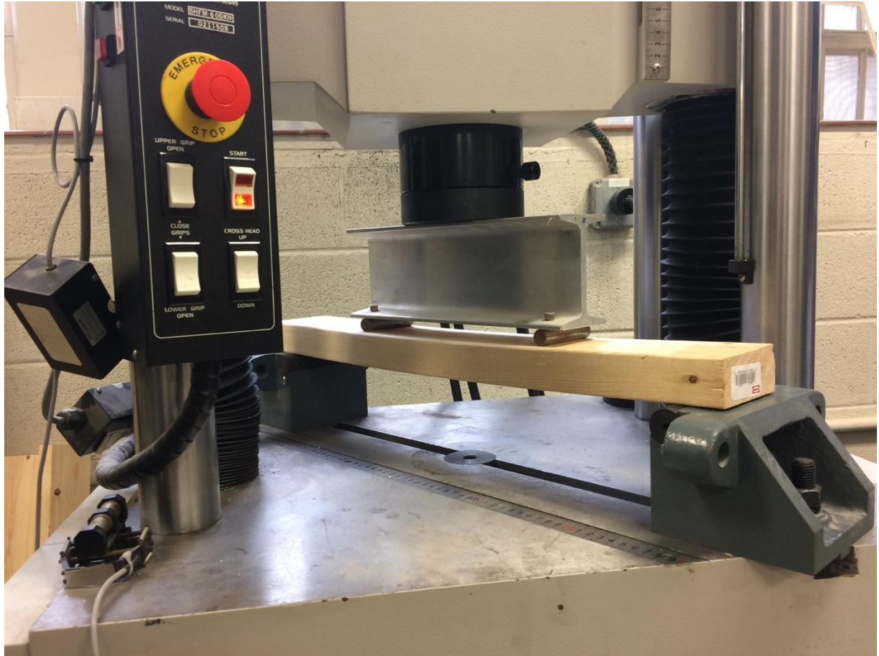
Figure 6 – Four-point bending apparatus
