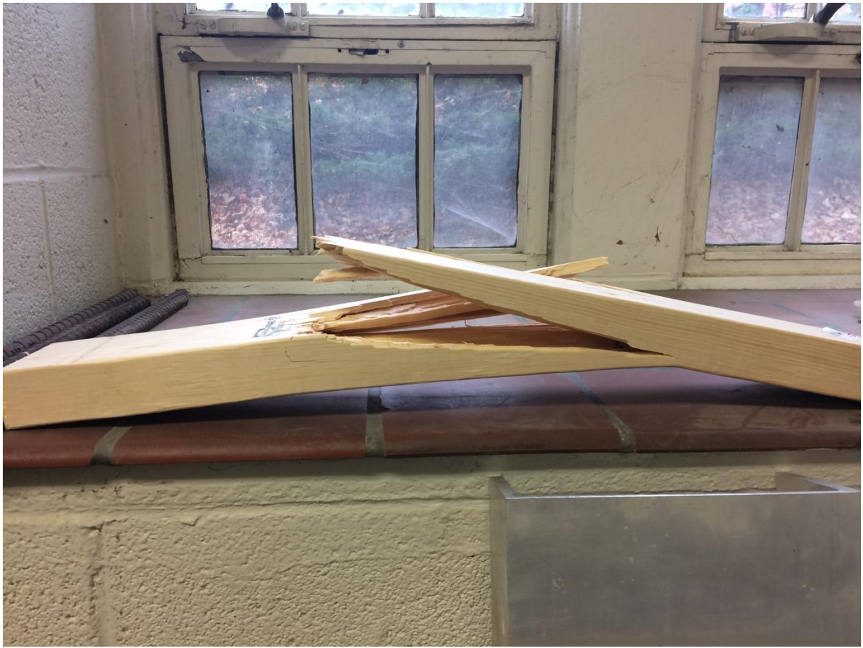
Figure 7 – Wood beam flexural failure
