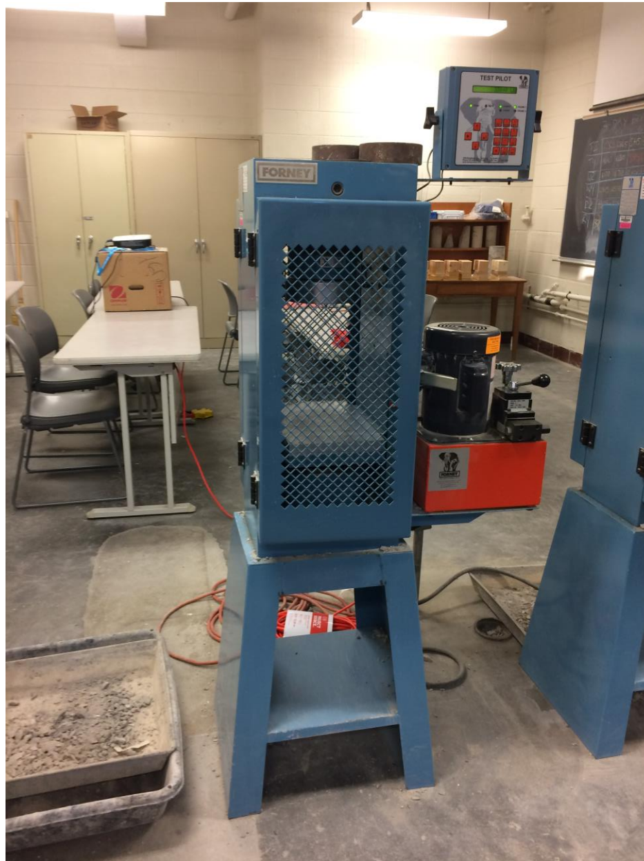
Figure 1 – Typical concrete cylinder testing machine
