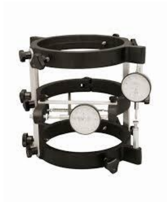
Figure 2 –Compressometer
