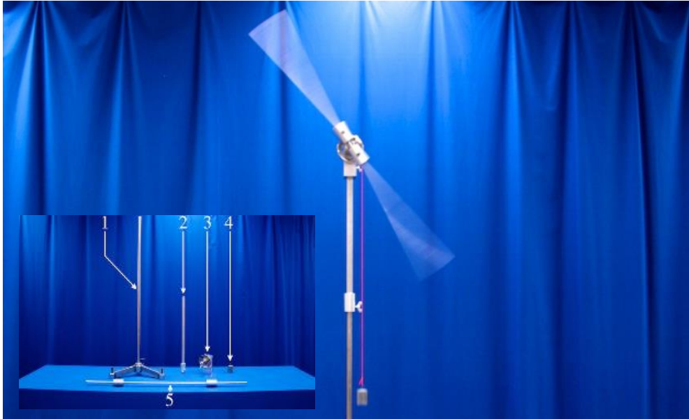
(Insert Figure 1) Figure 1: The extender connects to the top of the ring stand. The rotating assembly connects to the top of the extender and the torque bar connects to the rotating assembly. The weight is attached to a string which is wrapped around the axle of the rotating assembly. As the weight falls it will provide a torque on the axle which will result in the torque bar rotating. (Inset: 1. Large ring stand; 2. Extender; 3. Rotating assembly; 4. Weight; 5. Torque bar )
