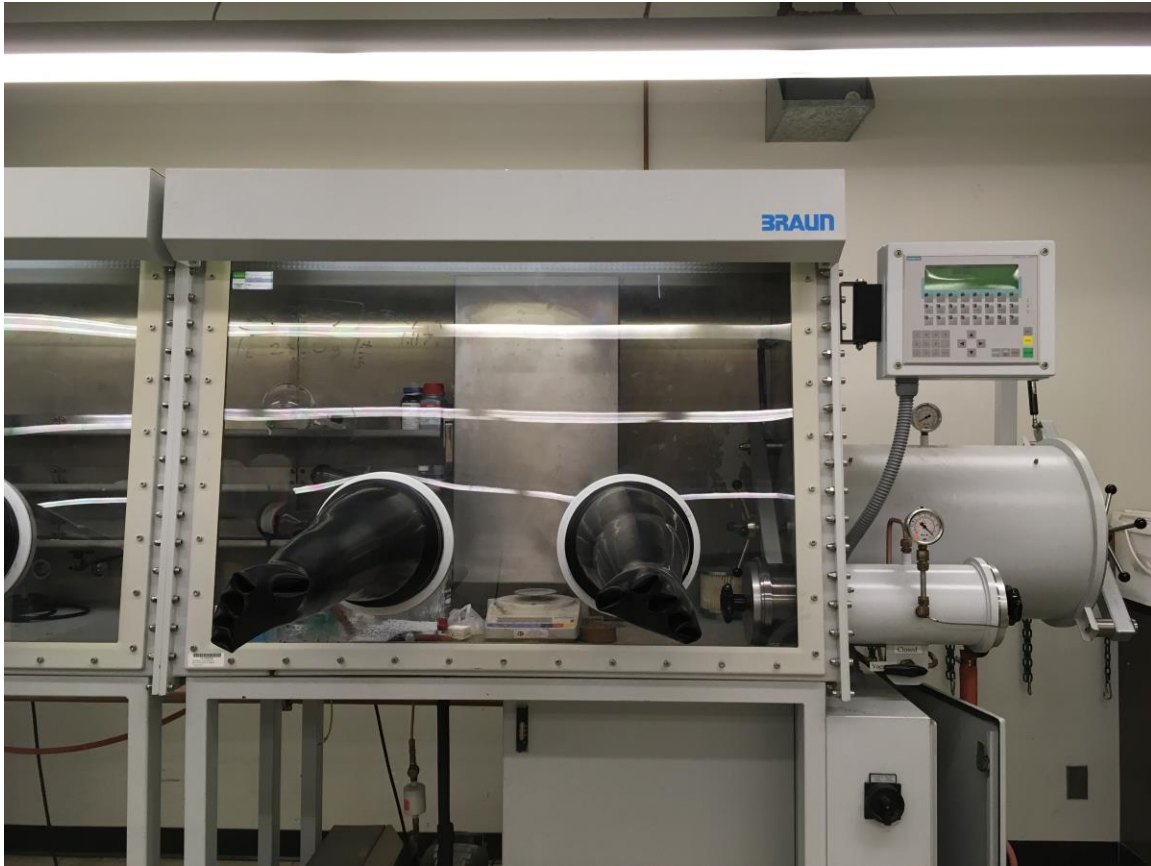
Figure 1. The glovebox, showing the main chamber, the gloves, the control panel, and the large/small antechambers.
